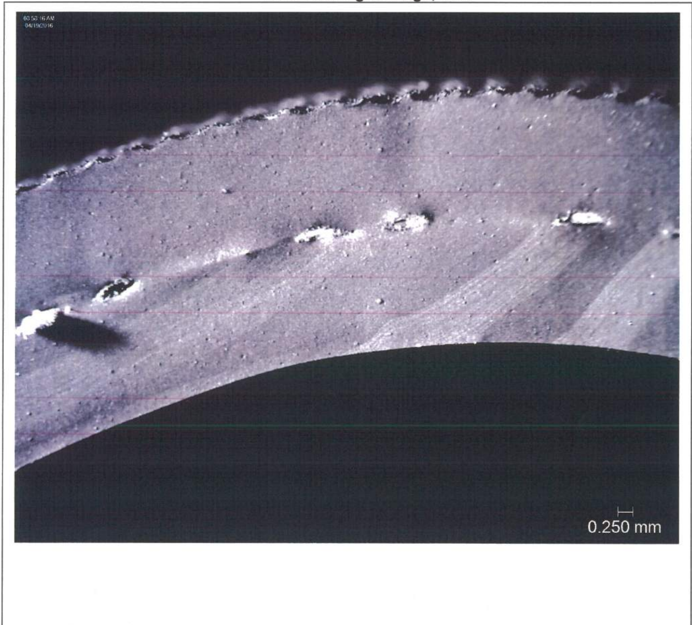
Figure C – Shore Rubber P/N 128187 Hose –78165A-3 After Brabolyzer Testing Reflected Light Image, 20X
