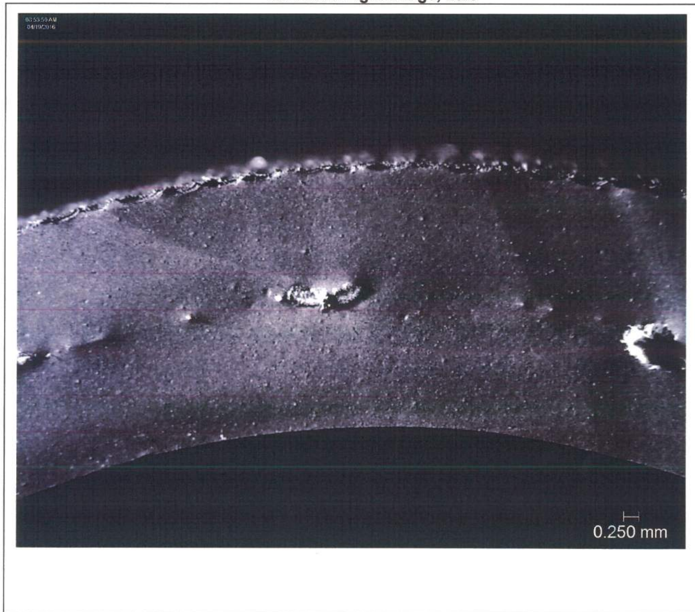
Figure B – Shore Rubber P/N 128187 Hose –78165A-2 After Brabolyzer Testing Reflected Light Image, 20X
