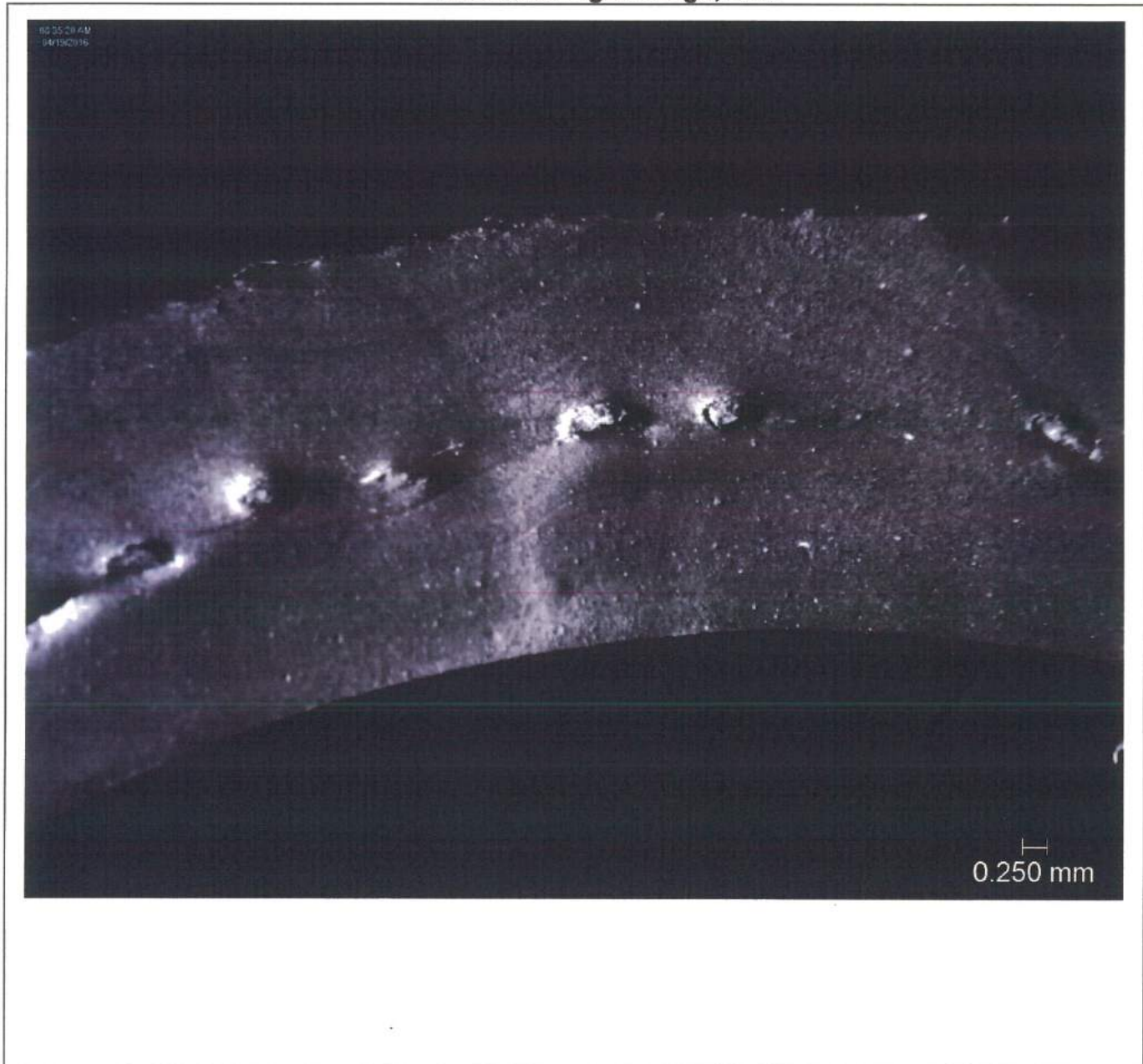
Figure D – Shore Rubber P/N 128187 Hose –79165A-1 After Brabolyzer Testing Reflected Light Image, 20X
