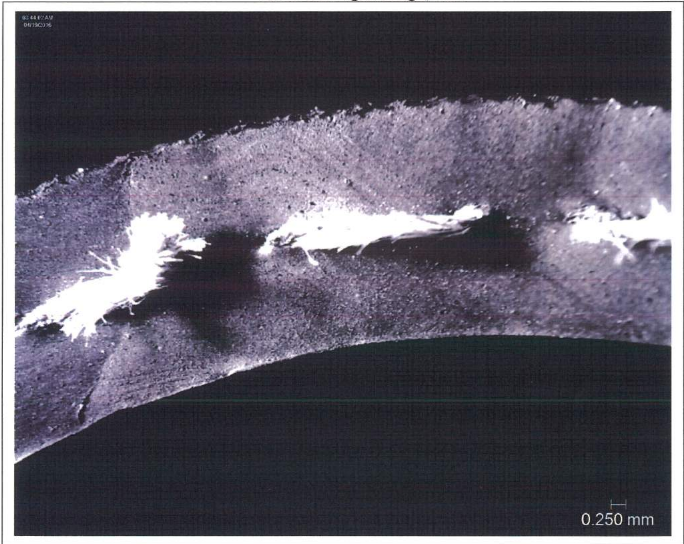
Figure F – Shore Rubber P/N 128187 Hose –79165A-3 After Brabolyzer Testing Reflected Light Image, 20X
